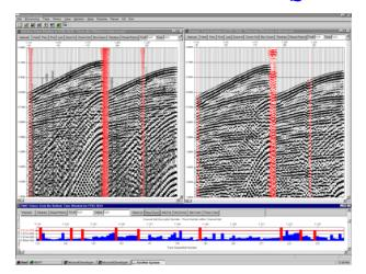
SeisNet's attribute analysis and display capabilities provide quality assurance of both the GeoRes/GSR recording system performance and seismic data integrity. Display image GIF files created by SeisNet may be distributed and viewed using the SeisNet QC Viewer utility, providing a convenient cost effective, environment friendly alternative to paper plots.
