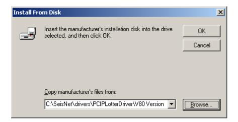
Browse to location of SeisNet PCIPlotter\V80 Version\PCIPLOTR.INF. Can be found under drivers directory on SeisNet CD or under c:\seisnet\drivers if loaded on the c: drive.
